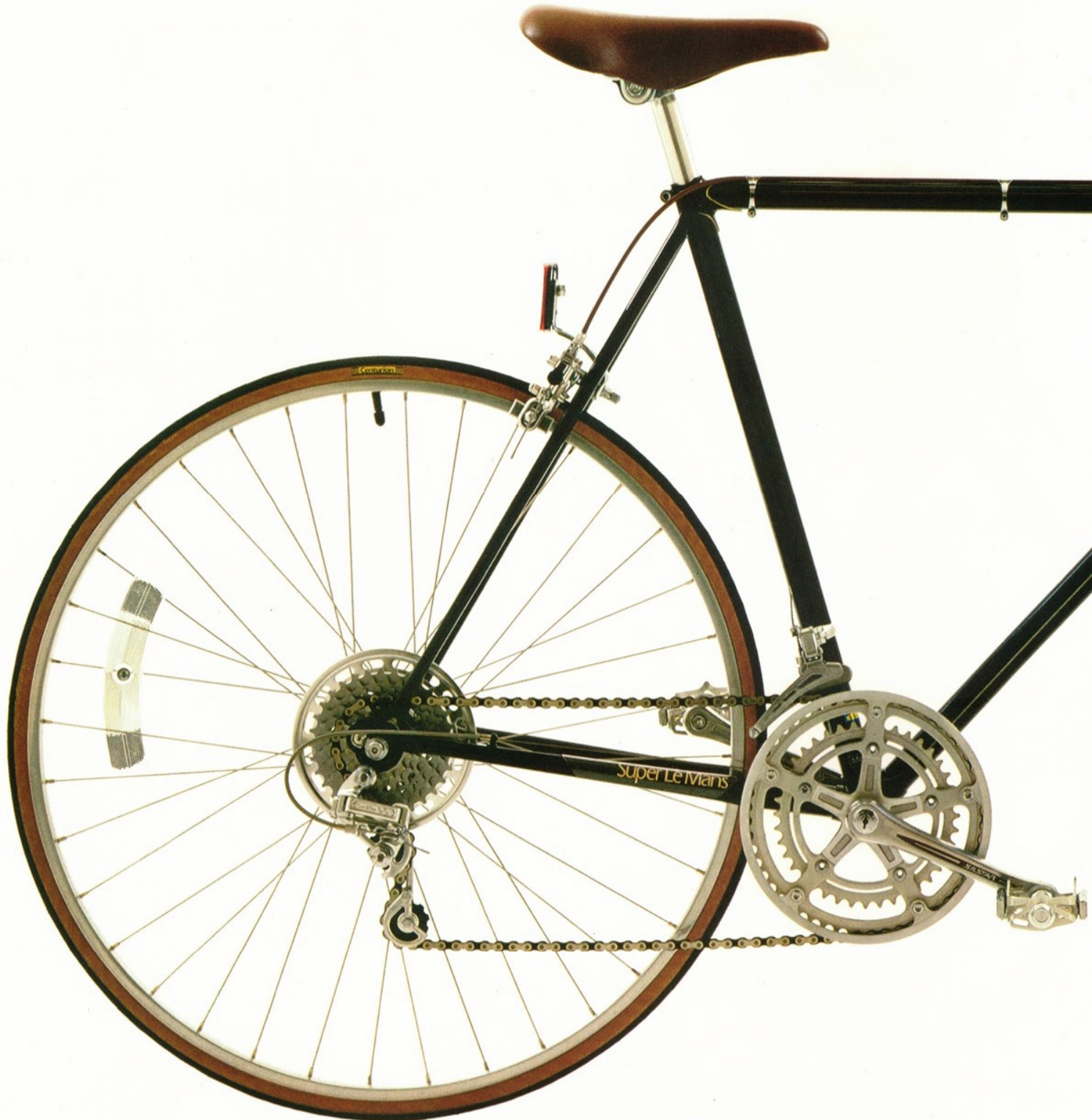
New Suntour Silver Ultra-Six freewheel and chrome plated chain. The 6-speed freewheel is as narrow as a normal 5-speed. Suntour new VX Derailleur system.
