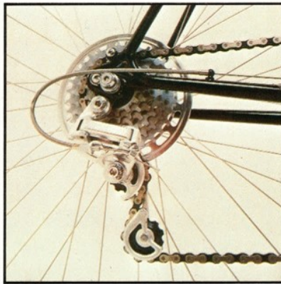
New Suntour Silver Ultra-Six freewheel and chrome plated chain. The 6-speed freewheel is as narrow as a normal 5-speed. Suntour new VX Derailleur system.
