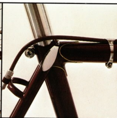
Chrome wrap-around seat stays. Special seat binder tube with chromoly dual allen head binder bolt for strong, positive locking. Brazed-on rear brake cable hanger with stop. Laprade type alloy fluted seat post, lightweight, extremely easy to adjust.
