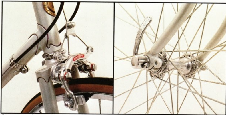
European-style fork design. Dia-Compe center pull brakes for positive, two-position stopping.
