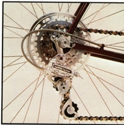
Suntour forged vertical rear drop-outs with dual mounts for rack and mud guard. Suntour Cyclone GT Derailleur system allowing chain removal from Derailleur cage without removing chain link. Suntour Tran-Z silver cluster and chain.
