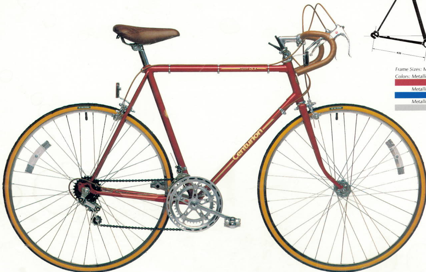
Convenient dual-position brake levers. Randonneur handlebars for more positions of comfort. Color-coordinated vinyl tape. Stem mounted shift levers.
