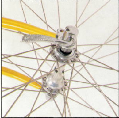
Sunshine Pro-Am small flange, quick release hubs with precision ground races for minimal friction. Stainless steel spokes.
