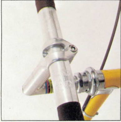
SR New Royal Extra Super Light stem. World Custom engraved handlebar with cloth tape for hand comfort, moisture absorption. Tange professional headset.
