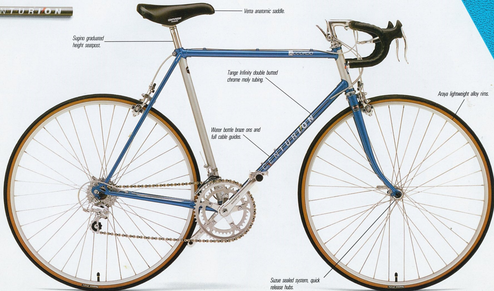
Rigid, Shimano Z brakes: Hidden cable aero brake levers with extension levers.
