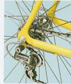
New, Sun Tour Sprint derailleur mounted to specially heat treated aluminum frame drop out.
