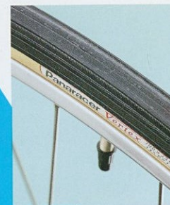
Araya 20c rims with Panaracer Vertex 115psi rated tires. 700C for easy conversion to tubular tires.
