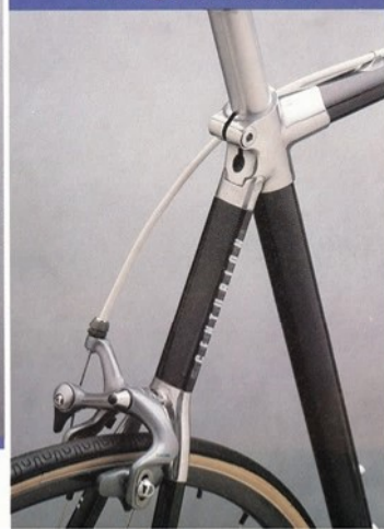
The Carbon's rear triangle uses a unique oval monostay for superior climbing characteristics.
