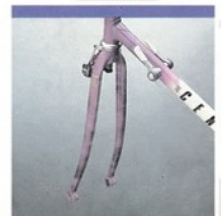
The '89 Le Mans uses a new, unicrown Chromoly fork.
